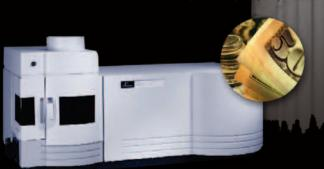
Assaying is performed with the state-of-the-art ICP-OES (Inductively Coupled Plasma-Optical Emission Spectrometer) one of the world's most sophisticated and accurate assaying units.
